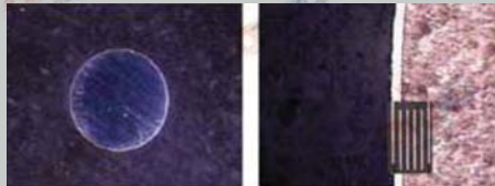
Cross-section of a NOVA pin under the microscope. The metallic layer is a thin layer on the pin surface.
